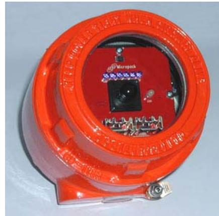
At the time, with the video imaging sensor (camera), all electronics and processing or decision making done internally in a single housing. It made for a very recognizable
