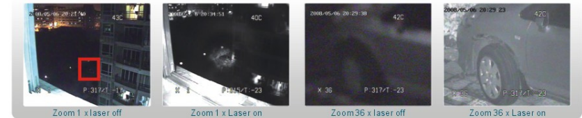
Outdoor Illumination <0.1 Lux The distance is about 100 meters between the Laser IR PowerView and the target with red mark
